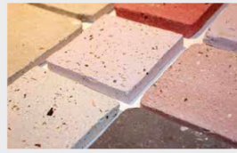
STAGE 2 Seashells are crushed and mixed with natural binders to form Seastone.
