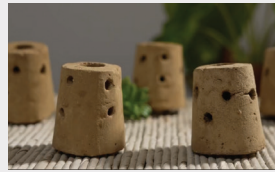
STAGE 3 The Seastone is molded to form the "Anchor"
